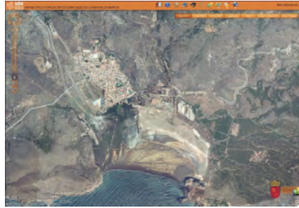
Figure 4. IDE. CARM. Portmán, 2011. Red delimits area filled with mining waste.
