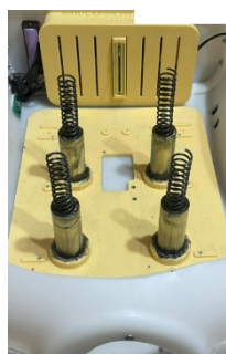
Figures 7 and 8. Mechanic system of resistance to compression (springs).
