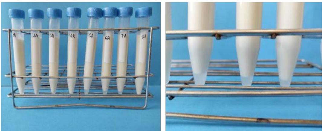
Figure 6. System used to determine the stability of emulsions by the static method. The phase separation can be seen in the lower part of the tubes, the cream, having less density, remains in the upper part.
