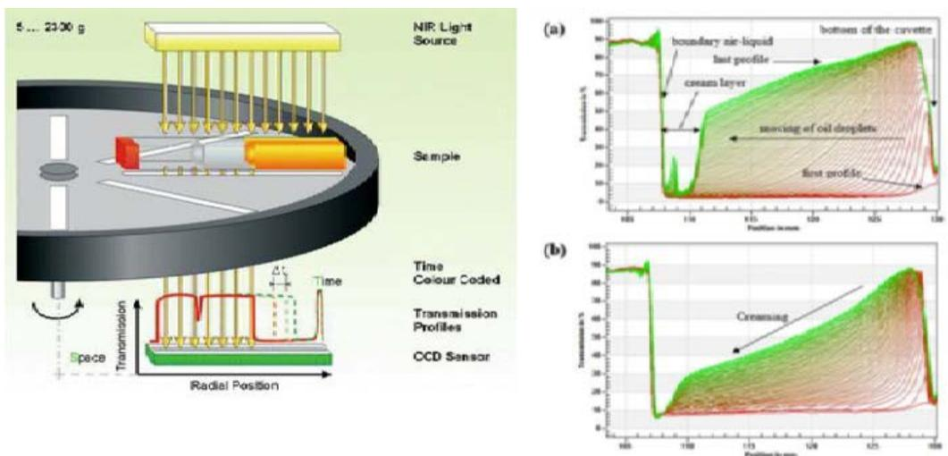
Figure 3. Schematic configuration and measurement principle of the LUMiSizer® analytical photocentrifuge (taken from Gross, Herrmann, Blech, Pinnapireddy, Garidel & Bakowsky, 2018), and transmission profiles of lecithin-stabilized emulsions (taken from Dammak & José do Amaral Sobral, 2018).
