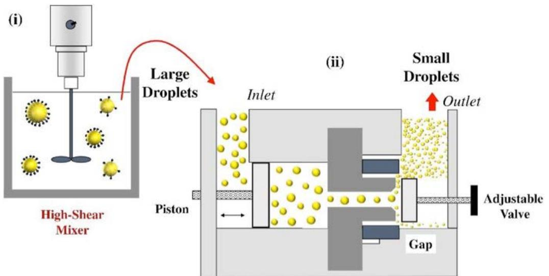
Figure 1.- Schematic diagram of the typical two-step procedure used to produce oil-in-water emulsions using a high energy method (i) a coarse emulsion is formed using a high shear mixer; (ii) a fine emulsion is formed by passing the coarse emulsion through a high-pressure valve homogenizer (taken from McClements & Jafari, 2018).
