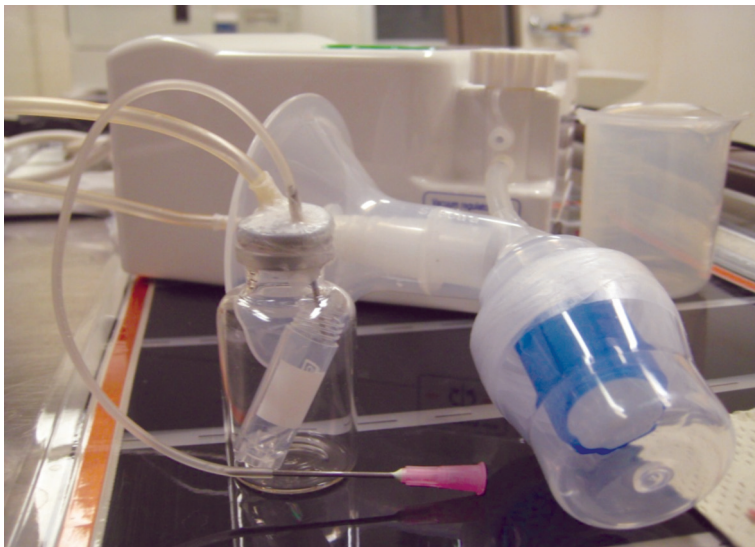
Figure 1. Modified electric breast pump and a glass vial for milk collection.
