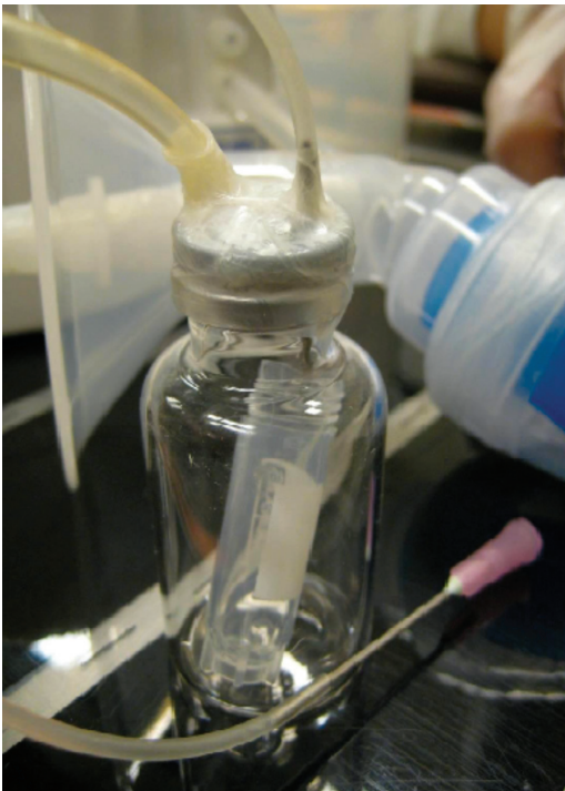
Figure 3. A glass vial containing a collection tube. The tube with larger diameter (left) is connected to the milking machine, and the tube with smaller diameter (right) is connected to an inverted needle serving as a suction cup.
